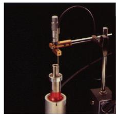
The Fotonic Sensor accurately measures the vibration amplitude of on ultrasonic welder tip at high frequencies and accelerations.
