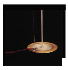
Two fiber-optic probes are used to measure surface displacement of a ceramic resonator. Fotonic probes are immune to electromagnetic interference (EMI) and operate effectively on a wide range of surfaces including nonmetalic materials, ceramic, glass, plastics, and composites.
