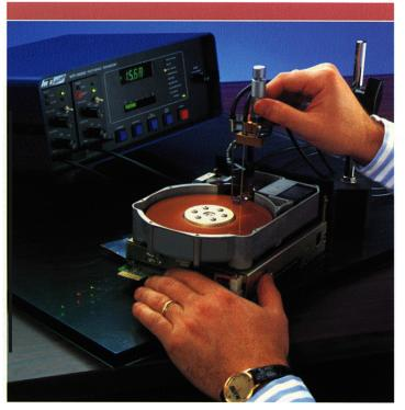
High-resolution, noncontact measurement of vibration and displacement
