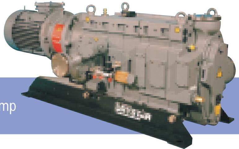
The GV600 dry pump extends the range of the currently successful GV Drystar® series. The pump is based on the well-proven claw mechanism but has an additional roots stage to enhance pumping speed in the working range. This makes it ideal for backing industrial diffusion pumps, without the need for an additional mechanical booster. The higher speed reduces time to crossover pressure.
