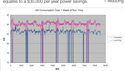
Actual kilowatt test results – with Alfa Laval's LKH-PF60 15% lower (in blue) compared to competition's less efficient pump (in pink)
