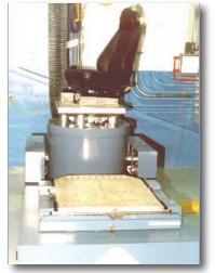
H560B-16 with slip table assembly, and guided head expander, testing an automotive seat track for squeak & rattle noise measurements and key life/durability
