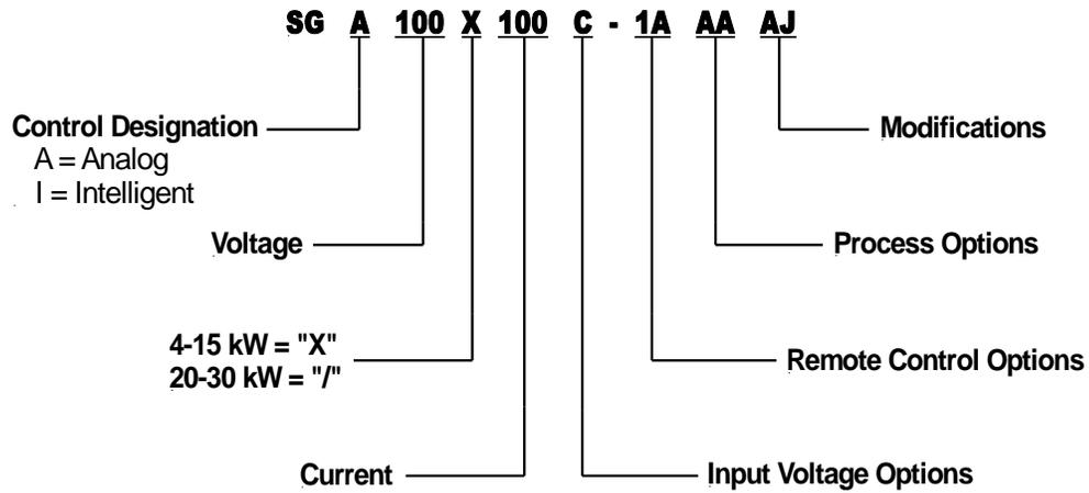
For units up to 999 V/999 A, voltage and current are represented in numeric format, e.g., "100" represents 100 V. For units at 1000 V/1000 A and above, the voltage and current are represented by the format "xKx", e.g., "1K2" represents 1000 V.
