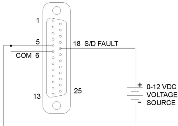
**Figure 3-21. Remote Shutdown Using DC Voltage Source**
