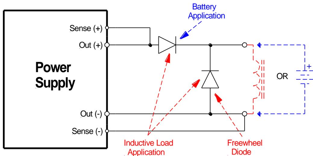
**Figure 2-1. Diode Connection**
