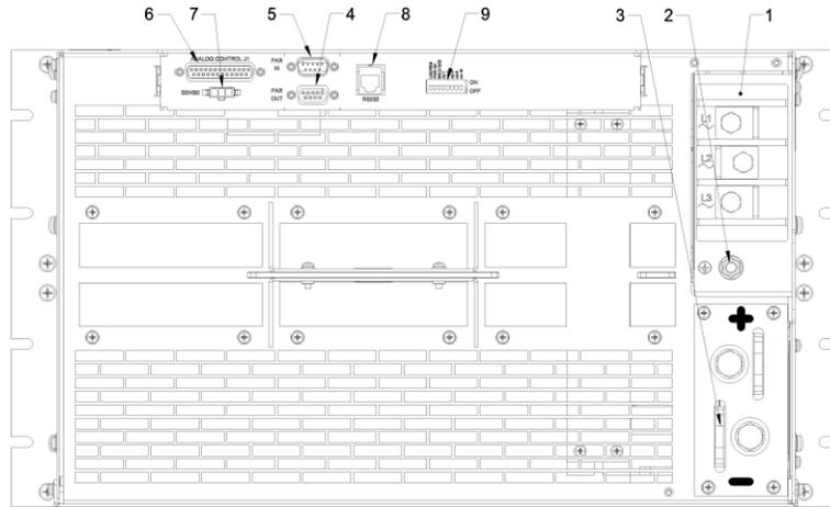
**Figure 3-8. Rear Panel Interface, Standard, 6U Models 20kW-30kW**
