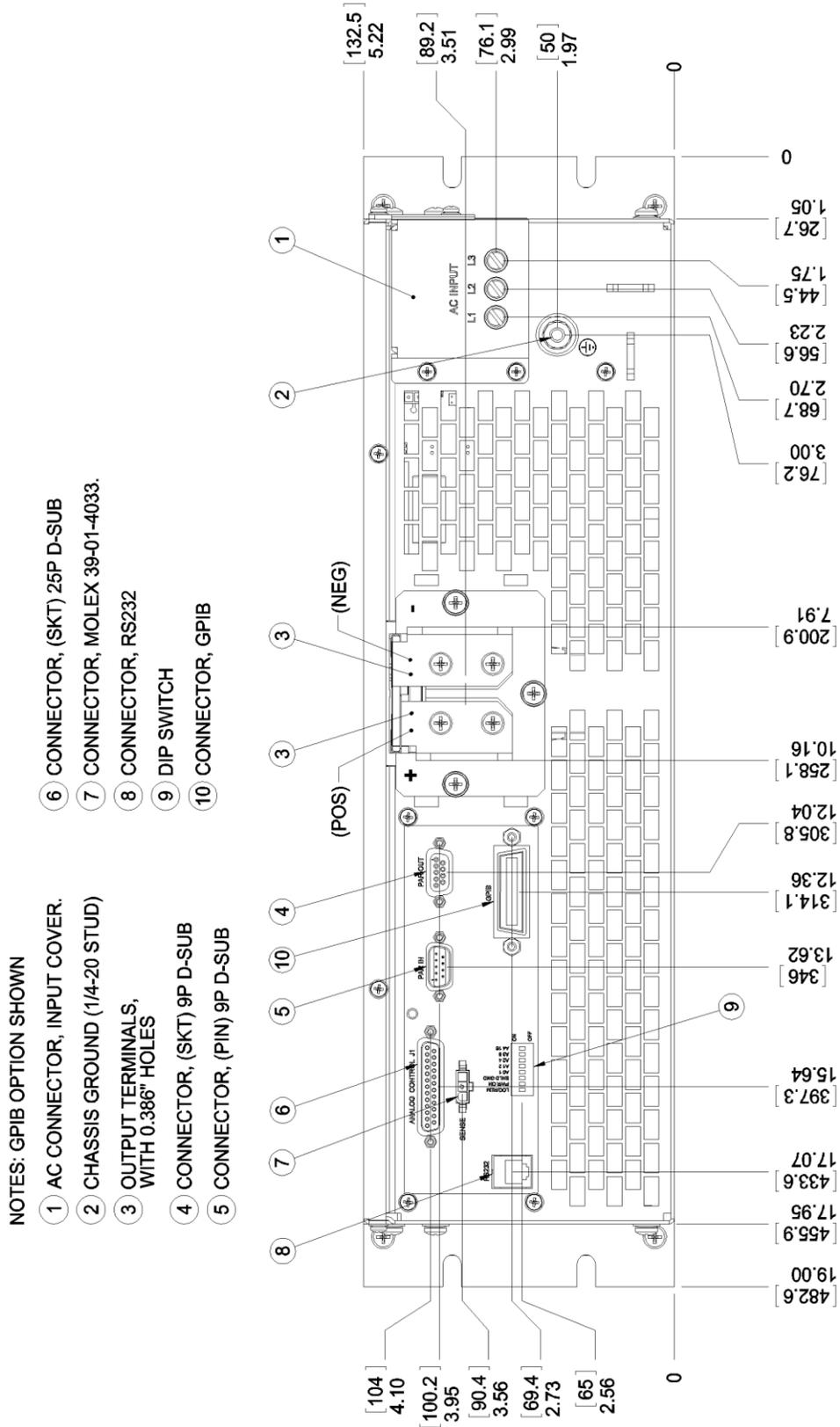
Figure 2-10. Rear Panel, GPIB Option, 3U Models 40V-600V
