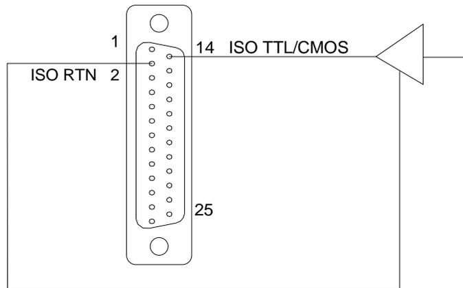
**Figure 3-20. Remote Output ON/OFF Using Isolated TTL/CMOS Source**
