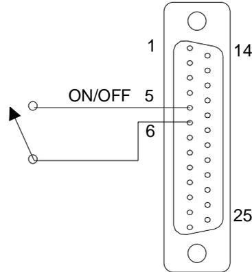
Figure 3-18. Remote Output ON/OFF Control by Contact Closure
